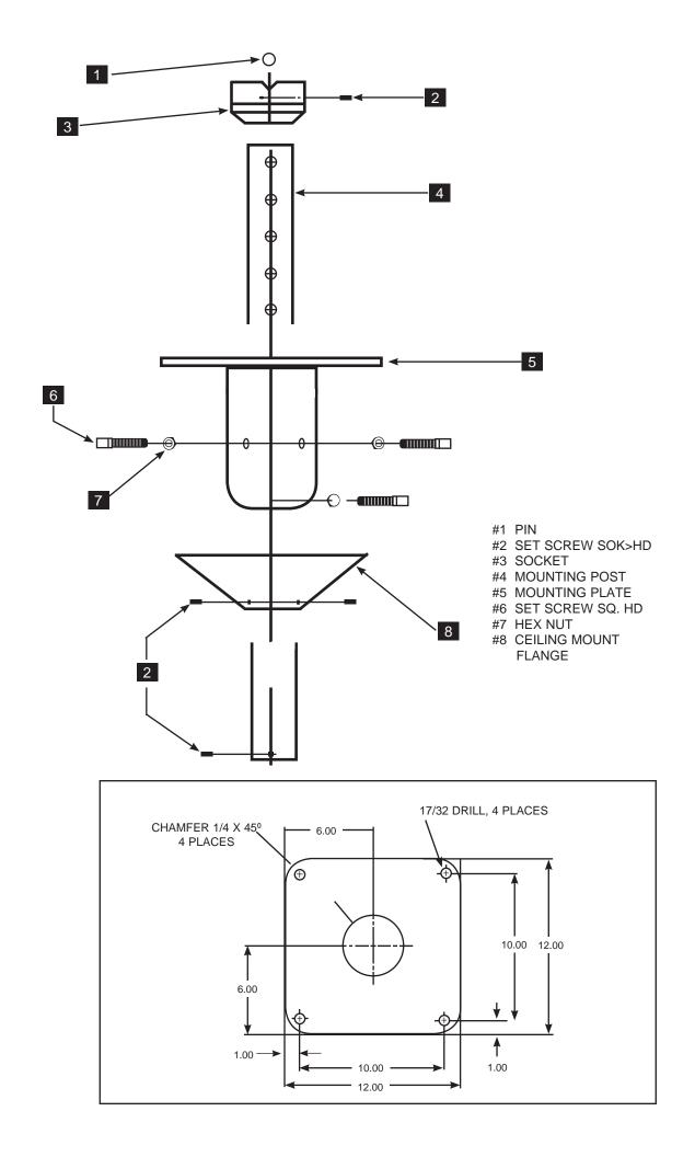
The next step is to level and secure the Mounting Post 4. To do this, loosen the six Set Screws 6 to allow the Mounting Post to tilt (it has a five degree tilt angle in all directions). Using a carpenters level held against the Mounting Post and the Mounting Post is plumb position, continue to tighten the set screws assuring that the column remains plumb. The six Nuts 7 may then be tightened against the Mounting Plate Assembly Tube.
